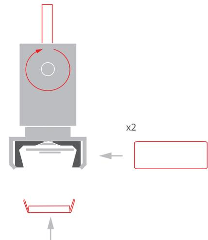
**5.** Install the W-KG ceiling fasteners. The fastener installation manual can be downloaded at [www.klusdesign.eu](http://www.klusdesign.eu). Place the power supplier next to the fastener and drill the ceiling to lead the cable to it.
